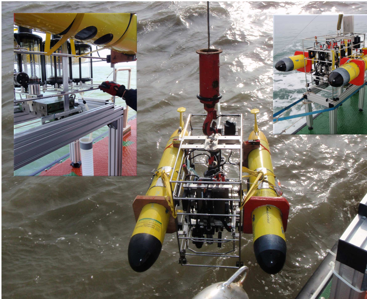
Figure III.6: An in-situ calibration frame, developed at HZG. The frame allows comparing the sensors of two gliders simultaneously, as well a suite of reference sensors (in the centre of the frame). Furthermore, the frame contains three vessels that can be used to collect water samples, controlled from a deck unit.
